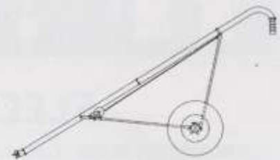
Optional remote load stand with wheels and winch (connects to pump with hose)
