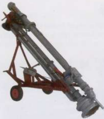
Super 120 with three point hook up and hand winch. Also available in two point trailer with hydraulic winch.
